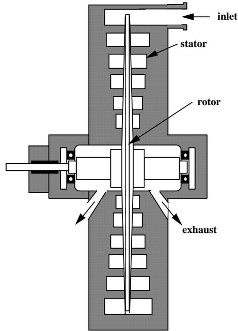
**Figure 10.2** Cross-section of a molecular drag pump using a spiral channel machined into the stator and a flared disc as a rotor.
