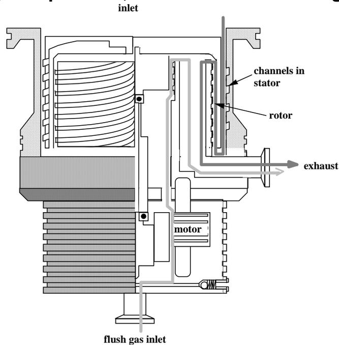
**Figure 10.3** A modern design for a molecular drag pump.
