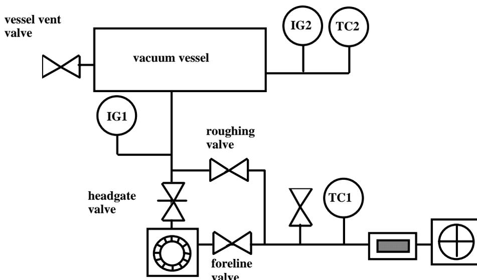
**Figure 10.5** .Typical turbomolecular vacuum pumped vacuum system configuration
