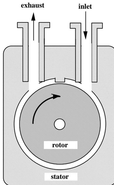
**Figure 10.1** Gaede's molecular drag pump of 1912.
