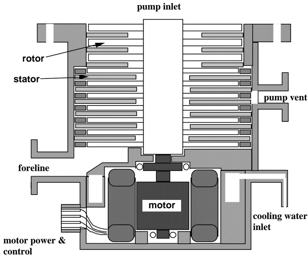
**10.4** Cross-section of an axial flow turbomolecular vacuum pump.
