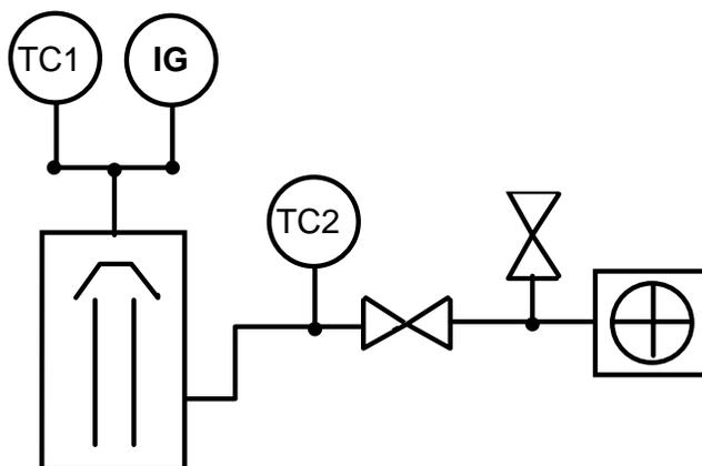
**Figure 7.3** Experimental set-up for measurement of DP base pressure.
