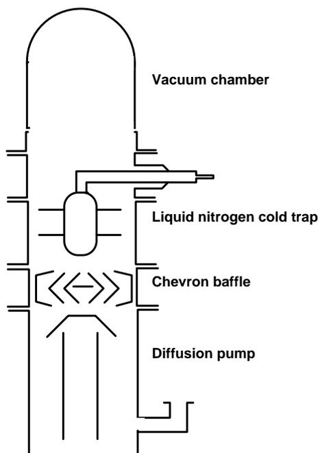
**Figure 7.1** Configuration of traps and baffles used on diffusion pumped systems.
