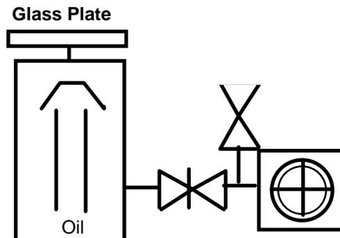
**Figure 7.2** Set-up for observation of DP backstreaming.
